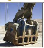
All Duratray Rubber Liners are reinforced with woven polyamide, offering abrasion resistance capabilities in addition to a wear life between 15,000 to 50,000 hours depending on application, abrasion, impact, and size distribution of the rock.
