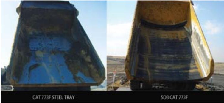
Due to different mineral conditions particularly in the process of overburden removal, several mines worldwide have experienced the problem of carry-back while reducing the load capacity of the haul equipment and preventing the mine from achieving payload targets.
