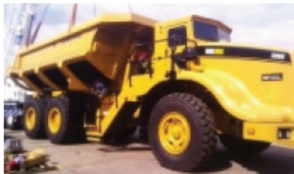
Haulmax 3900-D mine truck with Duratray dump body.
